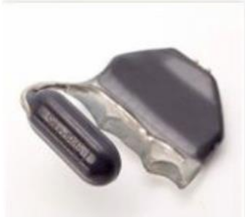
ITM hearing device inserted in-the-mouth
