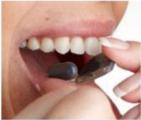
ITM hearing device inserted in-the-mouth
